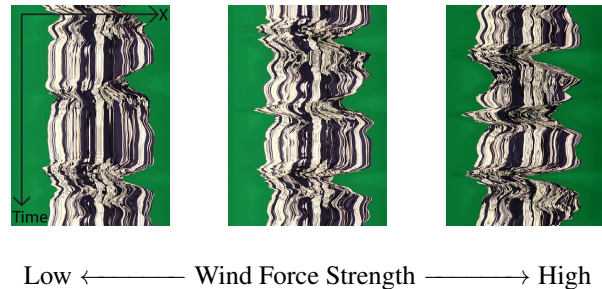
Figure 2. An example of a horizontal space \times time slice of the same fabric exposed to the three different strengths of wind from an oscillating fan. Note that the motion of the fabric appears very different under the different wind strengths.
