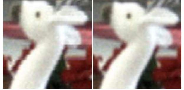
Figure 9. Barycentric reconstruction without (Left) and with (Right) sub-pixel precision estimation of micro lens center.
