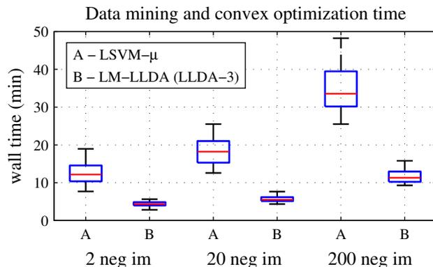
Figure 3. LM-LLDA spends one-third as much time on data mining and convex optimization compared to SVM- $\mu$  across various levels of negative image subsampling. The boxes span the 25th, 50th, and 75th percentiles of the time distribution over 20 classes.
