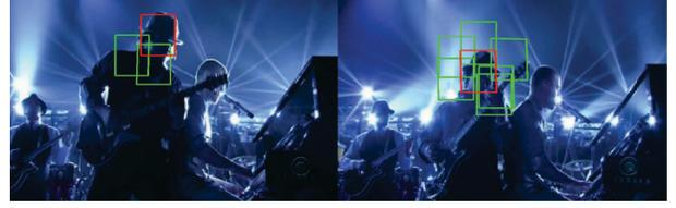
Figure 3. Examples of detected outlier tasks. The green bounding boxes denote the outlier particles and the red bounding box denotes the tracked target. The outliers are detected out of 400 sampled particles. There are two outliers in the left frame and six outliers in the right frame.
