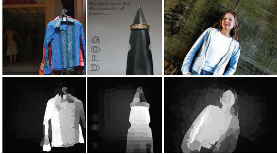
Figure 4. Examples in which the salient objects appear at the image boundaries. From top to down: input images, our saliency maps.
