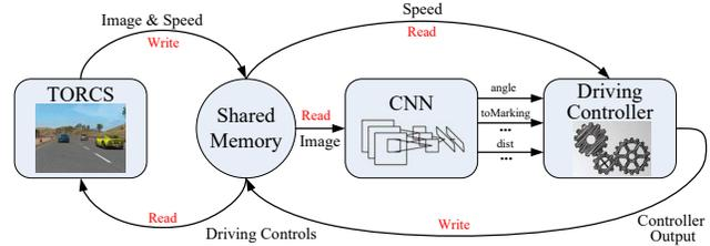
Figure 8: **System architecture.** The ConvNet processes the TORCS image and estimates 13 indicators for driving. Based on the indicators and the current speed of the car, a controller computes the driving commands which will be sent back to TORCS to drive the host car in it.
