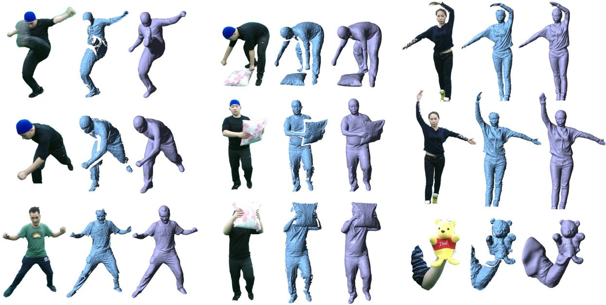
Figure 6. Results of our technique. For each result, we show a color image, the input depth and the reconstruction result. Notice that the color image is only for viewing the captured motion. It is not used by our system.
