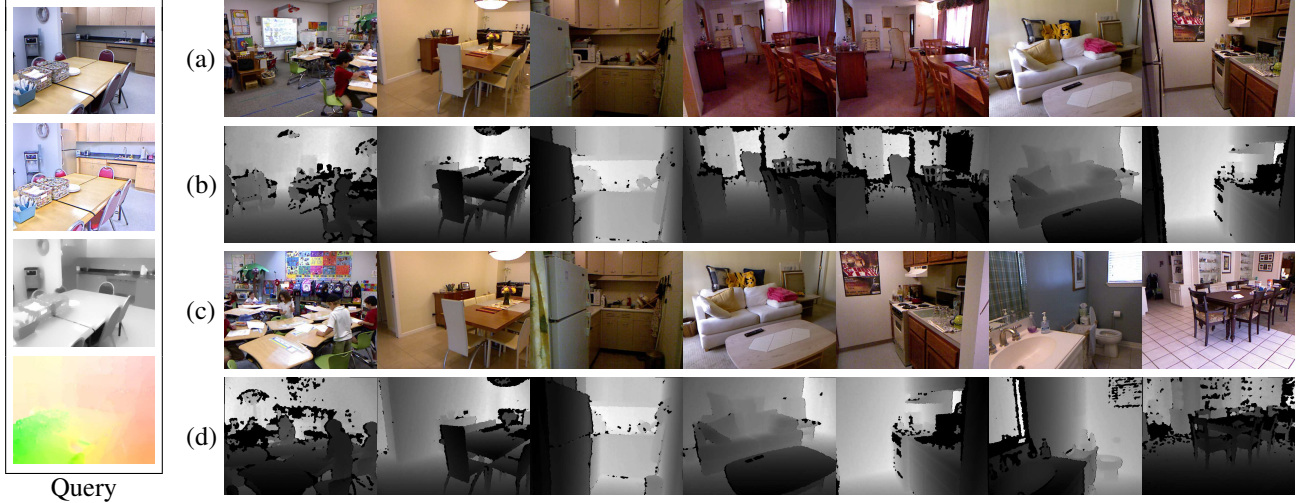
Figure 3. Candidate frame selection for a frame of the video in Fig. 1. The system chooses 7 candidate frames from the database. (a) shows candidates selected by pixel values and flow (original method) and (b) shows the corresponding depth maps. (c) shows candidates selected by pixels, albedo, shading, and flow, and (d) shows the corresponding depth maps. In (a) and (c), the images are sorted according to their matching scores in a descending order; the leftmost image is the best match for the query video (black pixels are unreliable measurements).
