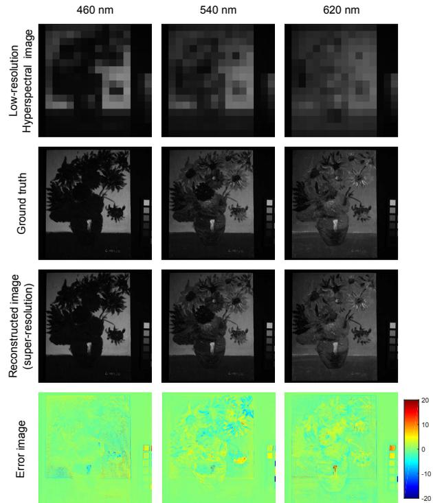
Figure 5. Spectral images of a painting from the CAVE database. Depicted are the spectral bands at 460, 540 and 620 nm. *Top row*: Low resolution input images. *Second row*: Ground truth. *Third row*: Reconstructed images from our method. *Bottom row*: Reconstruction errors in 8-bit range.
