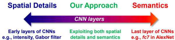
Figure 1. Convolutional layers of a typical CNN model, e.g., AlexNet [20], provide multiple levels of abstraction in the feature hierarchies. The features in the earlier layers retain higher spatial resolution for precise localization with low-level visual information similar to the response map of Gabor filters [4]. On the other hand, features in the latter layers capture more semantic information and less fine-grained spatial details. Our approach exploits the semantic information of last layers to handle large appearance changes and alleviate drifting by using features of earlier layers for precise localization.
