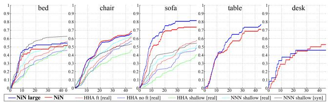
Figure 8. Pose estimation performance five classes in the NYUv2 [12] test set. We plot accuracy versus allowed angular error  $\delta_{\theta}$ . Our methods (NiN and NiN large - solid lines) outperform the state of the art results of Gupta *et al.* [4].
