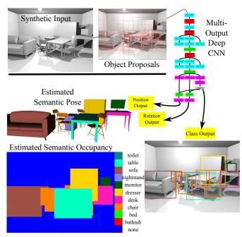
Figure 1. Overview of our approach. Normals for a scene are efficiently calculated using [7], proposals are generated using [8], and then fed through our synthetically trained CNN. Outputs are then consolidated using non-maximum suppression, leading to a scene class & pose heat map and a scene rendered with generalized models.
