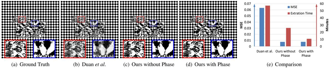
Figure 3. Comparison using synthetic data with ground truth (a). The result of [7] (b) is computed by capturing 40 images in the coarse level and 300 images in the fine level. It is blocky because of their square block assumption. Our CS-based approach (c & d) uses 320 images and shows better performance in terms of both accuracy and matte extraction time. The red and blue boxes show zoom in views.
