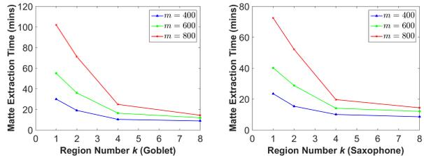
Figure 5. Effectiveness of using phase for accelerating matte extraction for two real objects: Goblet and Saxophone. Both results show that setting  $k = 4$  can lower the computation cost by several manifolds, especially when a large number of captured images ( $m$ ) is used. The benefit of further increasing  $k$  to 8 is limited.
