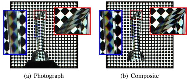
Figure 6. Handling dispersion. By processing the different color channels separately, our approach is able to render the rainbow phenomenon of the trophy. The greenish fringe around the checkerboard is due to chromatic lens aberration, which is not corrected in our experiment.
