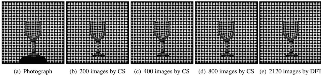
Figure 4. CS-based data acquisition on the Goblet object (under phase region  $k = 2$ ). As the number of images increases, the result of CS-based approach improves. With 400 images, the result is visually comparable to the conventional DFT, which requires 2120 images.
