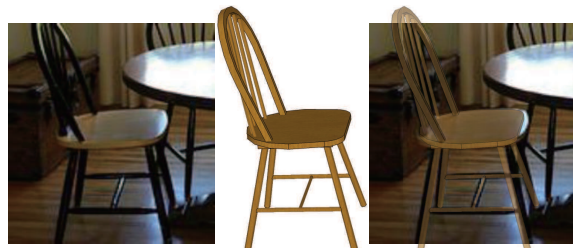
Figure 9. 3D model insertion. Recovered 3D viewpoint reduces search space of model retrieval.
