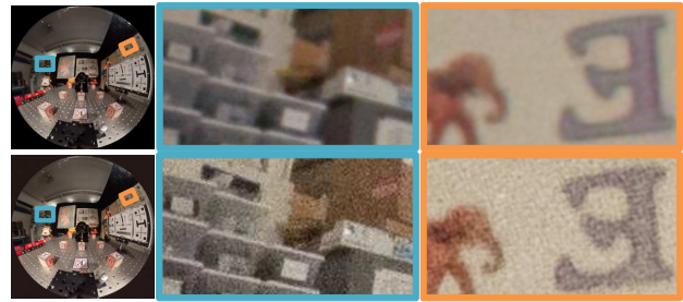
Figure 10: Comparison between EDOF image captured using our method (top row) and image captured with a normal camera using a stopped-down aperture (bottom row) for a scene brightness of about 50 lux. The former is captured with F2.8, 0.6 sec, and ISO100. The latter is captured with F11, 0.6 sec, and ISO1600.
