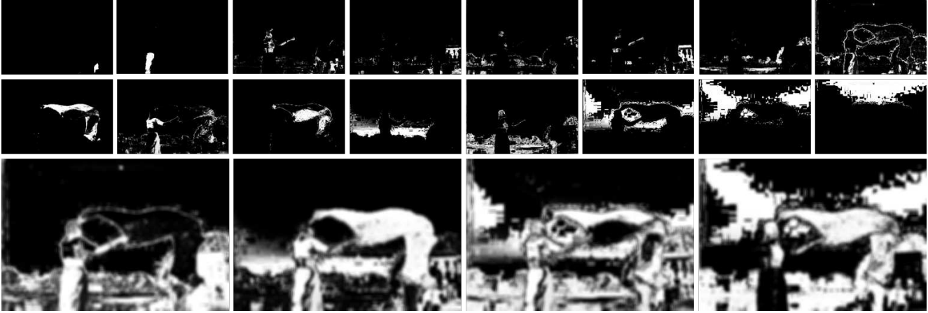
Figure 3. Initialization. The top two rows show pixelwise density defined by the 16 components of the Gaussian Mixture Model (GMM) learned from an input image. Images in the bottom row show a GMM-based initialization of the 4 dimensions of our embedding. Each image in the bottom represents the mixed density of 8 components of the GMM. Specifically, the first image in the bottom row records the mixed density of the 8 components in the first row; the second image in the bottom records the mixed density of the first 4 components in the top two rows; the third image in the bottom records the mixed density of the 1st, 2nd, 5th and 6th components in the top two rows; and the fourth image in the bottom records the mixed density of the 1st, 3rd, 5th and 7th components in the top two rows.
