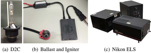
Figure 3. The 6000K D2C HID lamp (a) and its driving accessories (b). The input voltage is 12V and the power is 55W. The whole set costs about 30 USD, which is much more economical than the programmable ELS (c).
