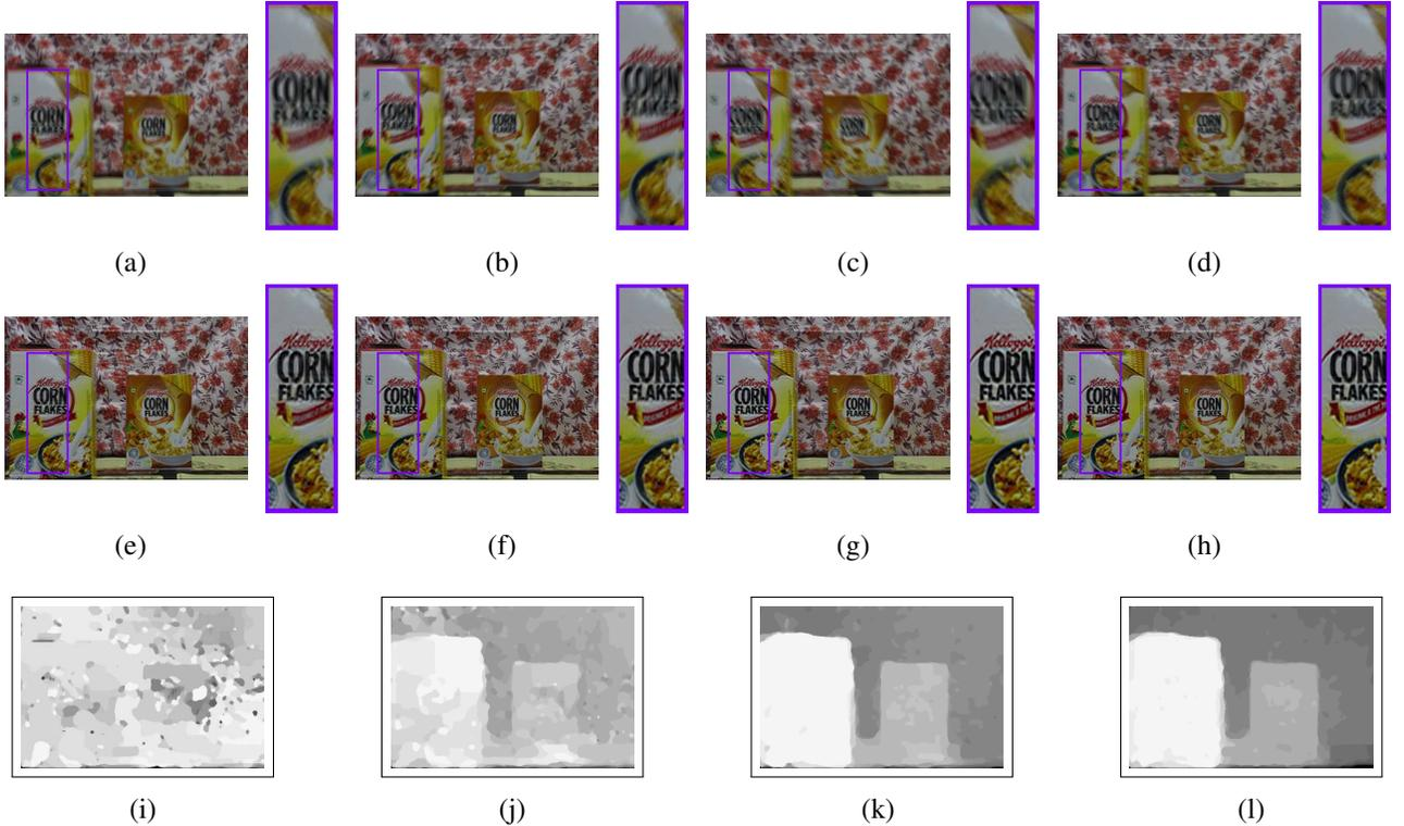
Figure 5. Real experiment: (a)-(d): Captured blurred images with zoomed-in locations marked. Estimated latent image and relative depth in (e) and (i): 1<sup>st</sup> iteration, (f) and (j): 2<sup>nd</sup> iteration, (g) and (k): 5<sup>th</sup> iteration, (h) and (l): 10<sup>th</sup> iteration.
