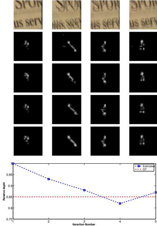
Figure 2. Iterative depth estimation at a point. First row: Blurred patches. Second row: Estimated PSFs for each patch. Third, fourth and fifth rows: PSFs generated using estimated TSF in the 1<sup>st</sup>, 3<sup>rd</sup> and 5<sup>th</sup> iteration respectively. Last row: Plot of depth update versus iteration number.
