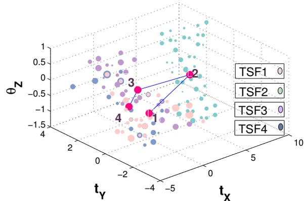
Figure 3. Ego motion: The camera poses corresponding to each of the blurred images are shown in same color. Red dot is the centroid of individual camera poses and blue line indicate the rough motion trajectory.
