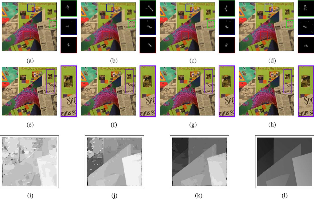
Figure 1. Synthetic experiment: (a)-(d): Generated blurred images with estimated PSFs at three different locations. Estimated latent image and relative depth in (e) and (i): 1<sup>st</sup> iteration, (f) and (j): 4<sup>th</sup> iteration, (g) and (k): 10<sup>th</sup> iteration. (h): Ground truth latent image. (l): True depth map.
