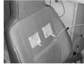
Figure 3: ECG measurements on driver's seatback in [45].
