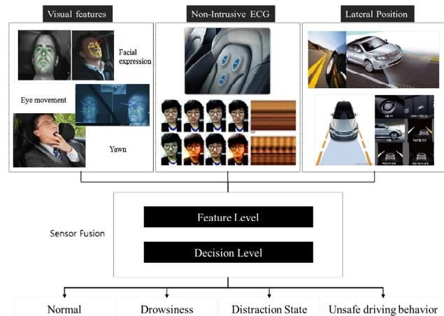
Figure 4: Hybrid measurement for detecting driver state.
