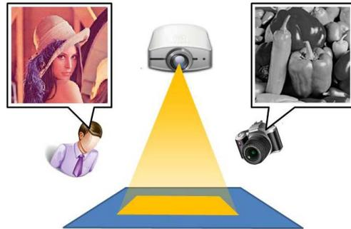
Figure 1. Multiplex image projection: Observers observe different images based on their spectral sensitivities.
