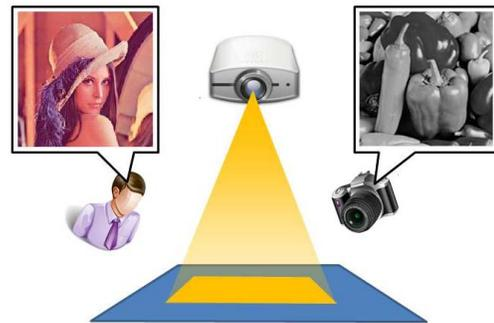
Figure 1. Multiplex image projection: Observers observe different images based on their spectral sensitivities.
