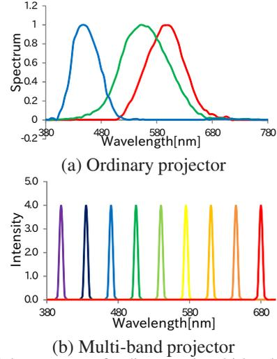
Figure 2. Light spectrum of ordinary and multi-band projectors
