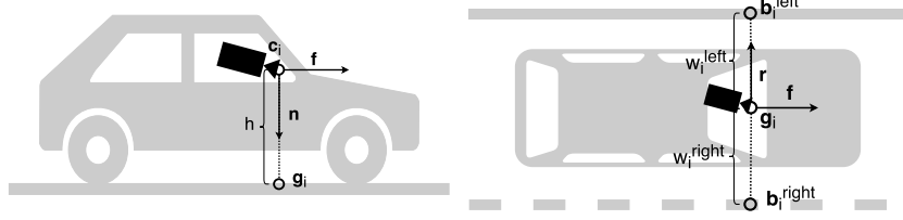
Fig. 2. Estimation of the lane border points \mathbf{b}_i^{left} , \mathbf{b}_i^{right} at frame i . \mathbf{c}_i is the camera position at frame i (obtained via SfM), \mathbf{g}_i is point on the road below the camera, h is the height of the camera above the road, \mathbf{f} is the forward direction, \mathbf{n} is the normal vector of the road plane, \mathbf{r} is the horizontal vector across the lane ( \mathbf{f} , \mathbf{n} and \mathbf{r} are relative to the camera orientation) and w_i^{left} , w_i^{right} are the distances to the left and right ego-lane borders.
