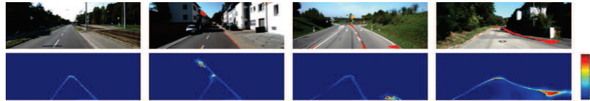
Fig. 4. Top: Original image and FP+FN area (red) generated by the initial network. Bottom: The image of absolute difference before and after the refinements by inter-link encoders. As noted from the heat maps, the initial false positive results are effectively suppressed and the originally missed lane pixels are well restored, as emphasized in warm color.
