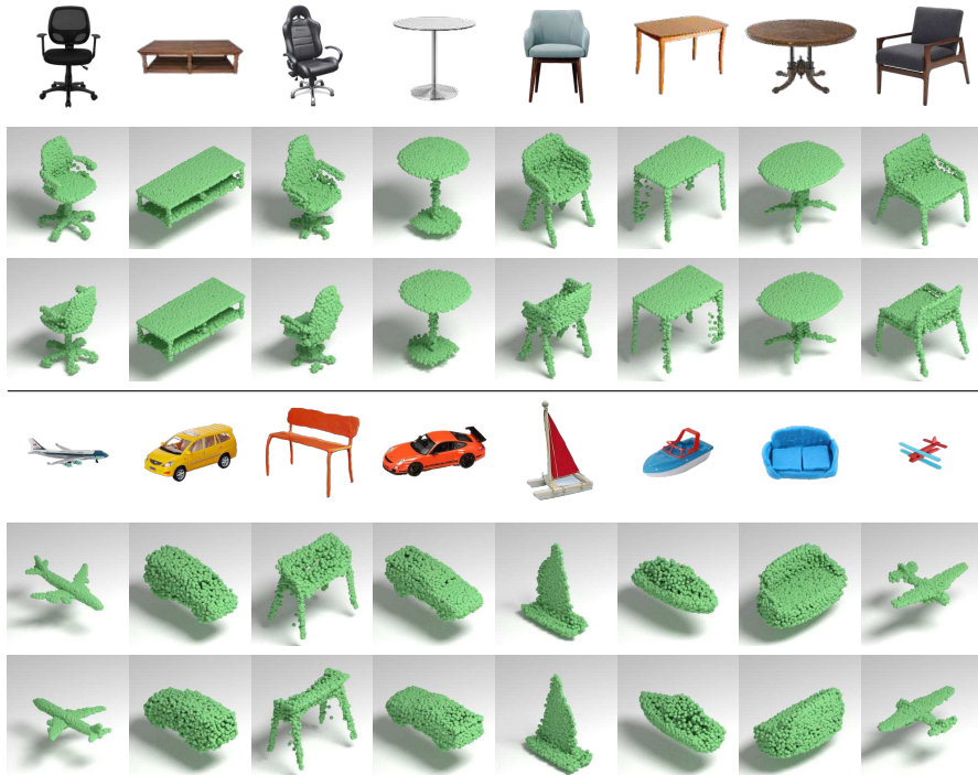
Fig. 6: Shapes generated by applying MRTNet on Internet photos of furnitures and toys. MRTNet is trained on the 13 categories of ShapeNet database (Table 2) . Note how the network is capable of generating detailed shapes from real photos, even though it is trained only on rendered images using simple shading models. For each output shape we show two different views.
