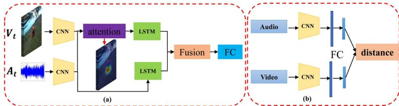
Fig. 3: (a) Audio-visual event localization framework with audio-guided visual attention and multimodal fusion. One timestep is illustrated, and note that the fusion network and FC are shared for all timesteps. (b) Audio-visual distance learning network
