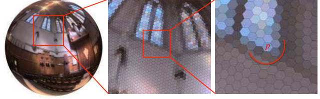
Figure 7: An example of a pixel passing the hexagonal 7-12 AST.
