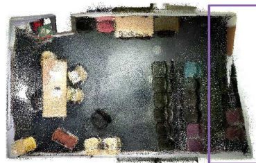
Figure 10: Failure case. In this trapezoidal room, our structural model incorrectly enforces walls on longer side of the room to be parallel, leading to intersections along shorter side (outlined).
