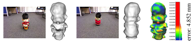
Figure 5. Canonical-pose result on a 360° sequence: KillingFusion reconstructs a complete, geometrically consistent model.
