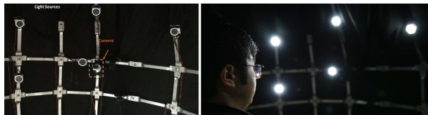
Figure 7: We constructed an acquisition system composed of 5 point light sources and a single DSLR camera.
