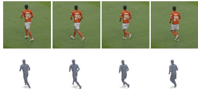
Figure 9. Depth estimation consistency for consecutive frames from 25 fps video, even the training data was captured at 1 fps.
