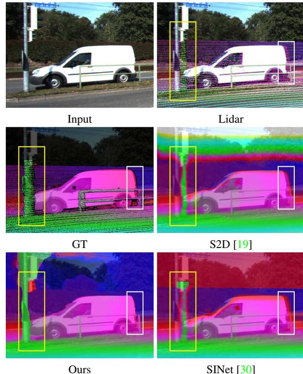
Figure 1. **Results on KITTI 2015.** We highlight the displacement error of Lidar points with bounding boxes. Lidar points are dilated for better visualization and we overlay our disparity maps to the colour images for illustration. Note the Lidar points for the foreground car and utility pole have been aligned to the background. Our method successfully recovers accurate disparities on tiny and moving objects while the other methods are misled by drifted and noisy Lidar points.
