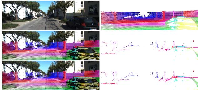
Figure 7. Gradually cleaned input Lidar points. From top to bottom, left column: left image, cleaned Lidar points at the 2<sup>nd</sup> epoch, cleaned Lidar points at the 5<sup>th</sup> epoch; Right column: raw Lidar points, error points find at the 2<sup>nd</sup> epoch, error points find at the 5<sup>th</sup> epoch. Note that the error measurements on the right car have been gradually removed.
