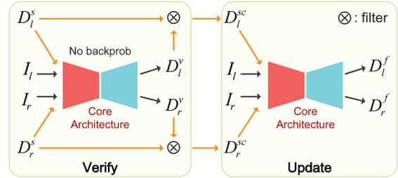
Figure 3. **The feedback loop.** For each iteration, the input stereo pair first computes initial disparities to filter errors in sparse Lidar points. At this stage, no *backprob* is taken place. So we call it the Verify phase. Then in the Update phase, the Core Architecture takes stereo pairs and cleaned sparse Lidar points as inputs to generate the final disparities. The parameters of the Core Architecture will be updated through *backprob* this time.
