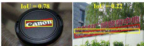
Figure 5: Red boxes: ground truths; Yellow boxes: detections. The corresponding angle is the same while the IOU diverges hugely.
