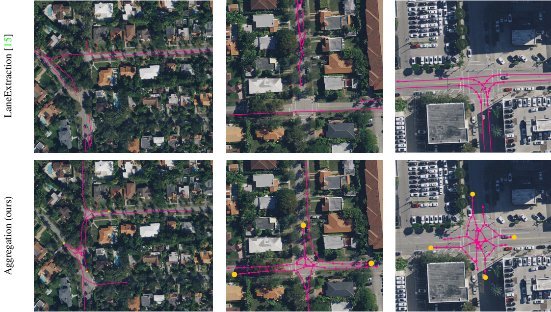
Figure 6. Qualitative results on the Full-LGP task. We visualize predictions of LaneExtraction [15] (top row) and aggregated LaneGNN predictions (bottom row). Our model is initialized at poses using predicted lane direction masks of LaneExtraction (indicated with yellow circles). Best viewed zoomed in.
