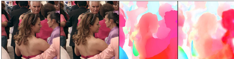
Fig. 7: An example of the estimated optical flow, left to right: two consecutive frames used for estimation, FlowNet2 results, our decoder output \hat{\mathbf{f}} . Note that the flow produced by our model is decoded from a compressed latent, and is trained to maximize total compression performance rather than warping accuracy. See Appendix B for license information.
