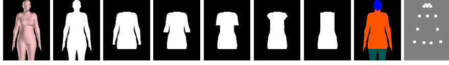
Fig. 5. 2D cloth mapping process to the reference SMPL silhouette. From left to right: standard body model and its silhouette, matching masks for long-sleeve, half-sleeve, short-sleeve (half-elbow and quarter elbow respectively), sleeveless clothing categories, and the standard model inputs for generating matching masks with SGN & MGN.
