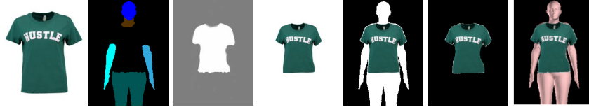
Fig. 7. Example of 2D cloth matching for 3D reconstruction. From left to right: Input cloth image, target body segmentation generated by SGN for standard body model, cloth matching mask generated by MGN, cloth texture after 2D matching and overlapped on SMPL silhouette respectively, 3D reconstructed cloth and overlaid on SMPL model respectively.
