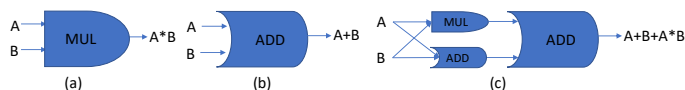
Fig. 2. Illustration of our feature fusion block add-multiply-add ( AMA ), which is more expressive than either add or mul , but does not increase feature dimension like concat .
