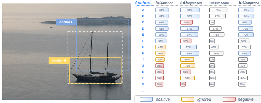
Fig. 2. Illustration of different anchor matching strategies for the boat image resorting to IoU_{anchor} (static), IoU_{regressed} ( Localize to Classify ) and IoU_{amplified} ( Classify to Localize ). Anchors A-M are predefined anchor boxes around the boat in the picture (only F and H are visualized as examples). Better viewed in colour.
