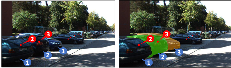
Fig. 1. An example of center-point-based object representation. The red points in the left sub-image are the projected 3D center of the objects on the 2D image. The numbers in the blue text box represent the “ID” of vehicles. The red points are the projected 3D vehicle centers onto the 2D image plane. The number in the red text boxes represents which vehicle that the center point belongs to.
