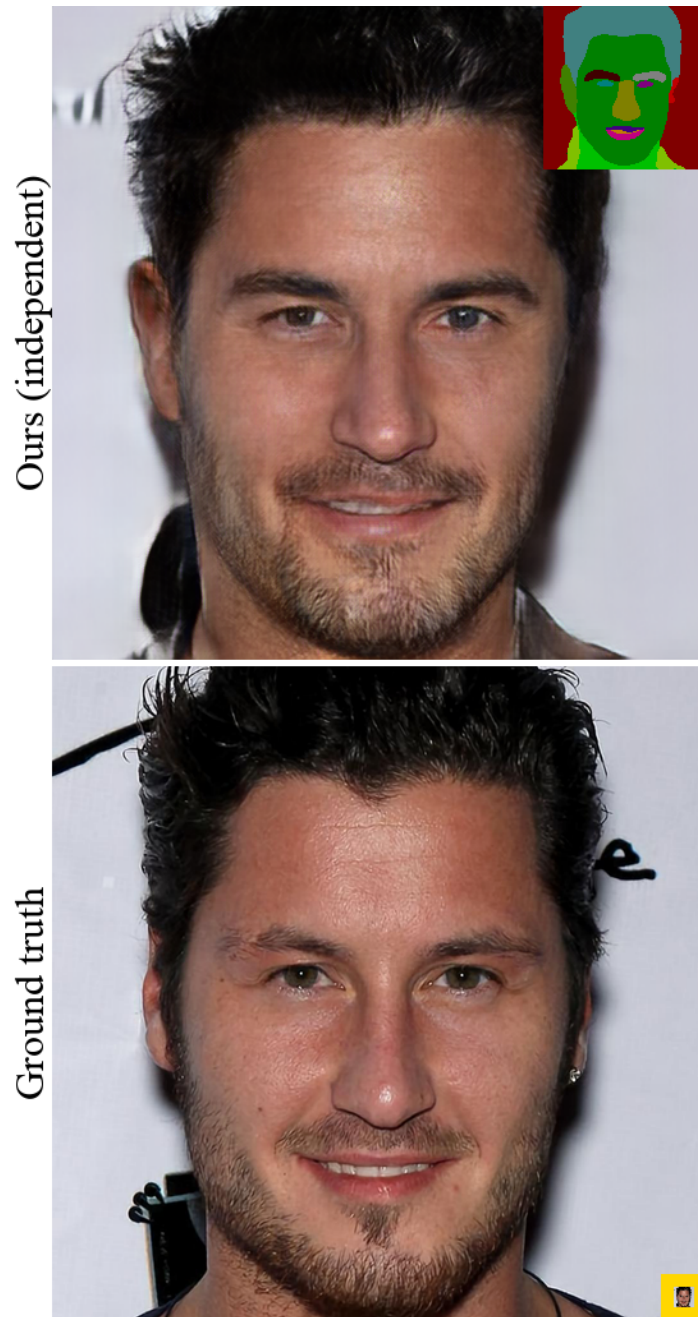
Fig. 14. Extreme Super-resolution (1). This figure shows a larger version of the extreme super-resolution example in the main paper. The yellow image in the bottom right is the low-resolution input image, which is upscaled 32\times .
