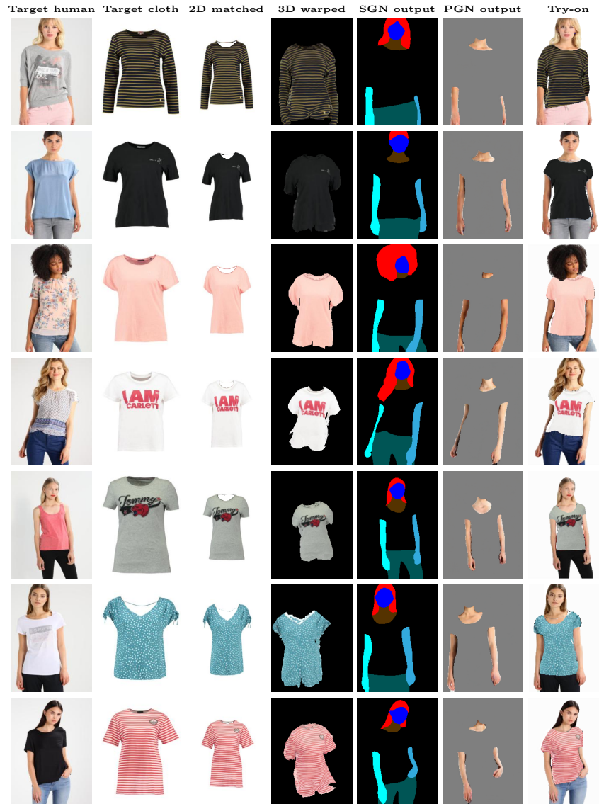
Fig. 4. Sample results of our CloTH-VTON, showing step-wise results from each stage (See Section 2.2). The first two columns are the inputs, then the corresponding results from the consecutive steps, i.e., 2D cloth matching, 3D reconstruction and deformation, Segmentation Generation Network (SGN), Parts Generation Network (PGN), and final fusion.
