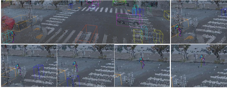
Fig. 1: A subsampled pose sequence in Waymo showing the SPL agent cutting corners and choosing to avoid the crosswalk. This kind of imperfect but plausible traffic behaviour would not be modelled by classical planning methods. To the top left : it can be seen that no cars are approaching the pedestrian. The pedestrian continues to the left once on the pavement.
