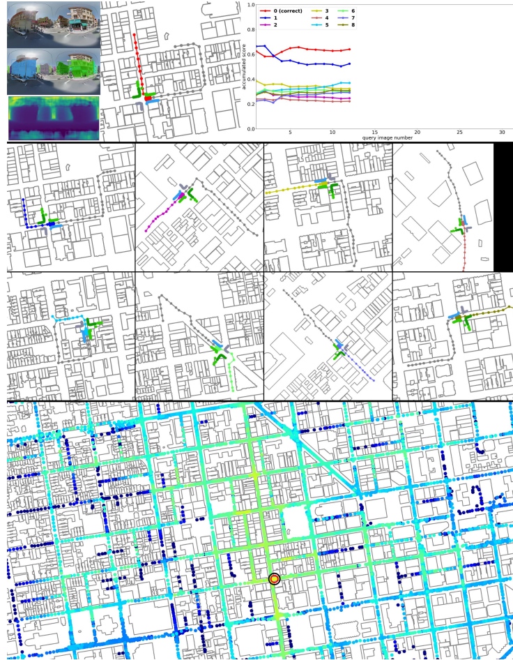
Fig. 3. This figure shows a single frame from the supplementary video, which illustrates the qualitative results of the trajectory level localization. The video shows the progress of the trajectory localization accuracy while increasing the length of the trajectory (from 1 to 32). The top left column of three images shows the most recent query image within a trajectory, corresponding segmentation labels and depth values. The middle image of the top row illustrates the query trajectory where the red color shows already traveled frames. The final image in the top row shows the graph, which plots the similarity score between the query trajectory and (i) its correct location (red), (ii) the top-2 retrieved trajectory (blue) and (iii) 7 random alternative trajectories from the map. The second and third rows of the figure the alternative trajectories (note that blue trajectory is always second best). The last row plots similarity score for each Google StreetView map location of the best matching trajectory which ends at that point. The similarity is encoded using "jet" colormap (i.e. red corresponds to high similarity and blue to low similarity). The black circle marks the correct ground-truth location and the red circle marks the current most likely endpoint of the trajectory.
