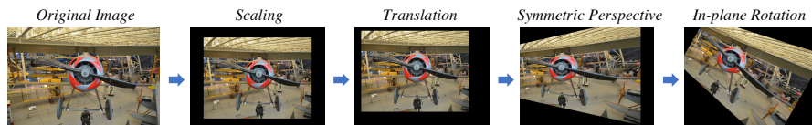
Fig. 1. The visualization of homography sampling. The input image is sequentially transformed by Scaling, Translation, Symmetric Perspective, and In-plane Rotation.
