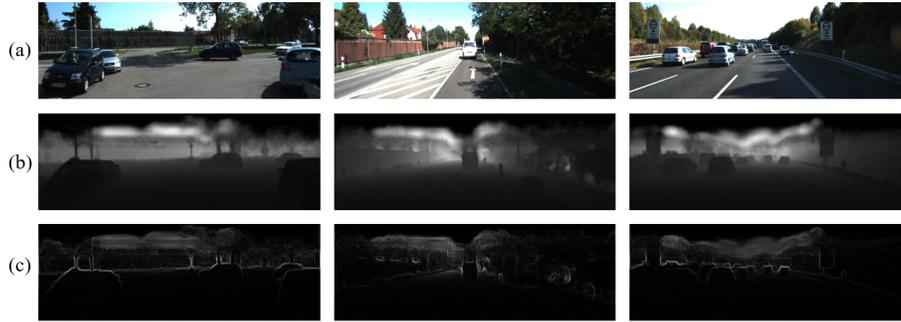
**Fig. 5. The middle results of CGM.** (a) The reference color images, (b) first depth maps form stage 1, and (c) feature maps after applying the Sobel filter. (c) Sobel-filtered features have high intensity on the pixel of object boundary and distant area, meaning that the Sobel filter is an essential factor in CGM to represent the characteristics of each modality.
