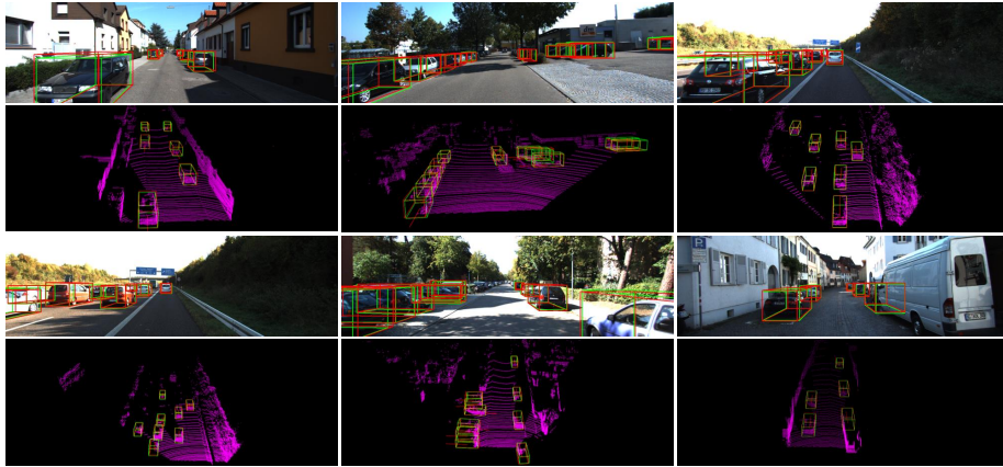
Fig. 4. Qualitative results on KITTI val set. The predicted bounding boxes and ground-truth bounding boxes are shown in red and green, respectively, and we project them back onto the color images for better visualization.
