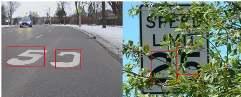
Fig. 5: Sample detections on worn-out and partially occluded speed limit postings using Faster-RCNN trained on CaltechFN.
