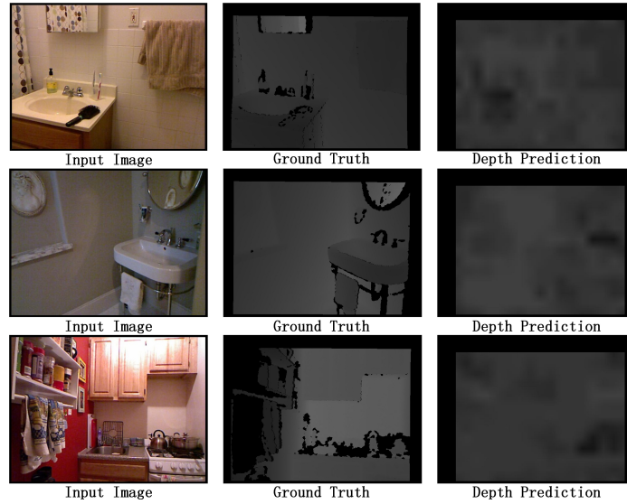
Fig. 2: Visualization of depth prediction, compared with RGB images and ground truth.
