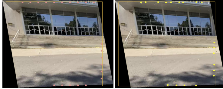
Fig. 3. In this example, source and target images are represented using a bitmap form and a rectangle. (Left) Control points are uniformly sampled at the boundary of the overlapping area. (Right) Points are adjusted to high gradient positions for better alignment around structural regions. Note that control points are used to warp the outer region of a source image, and the points in the bottom left corner are unnecessary.
