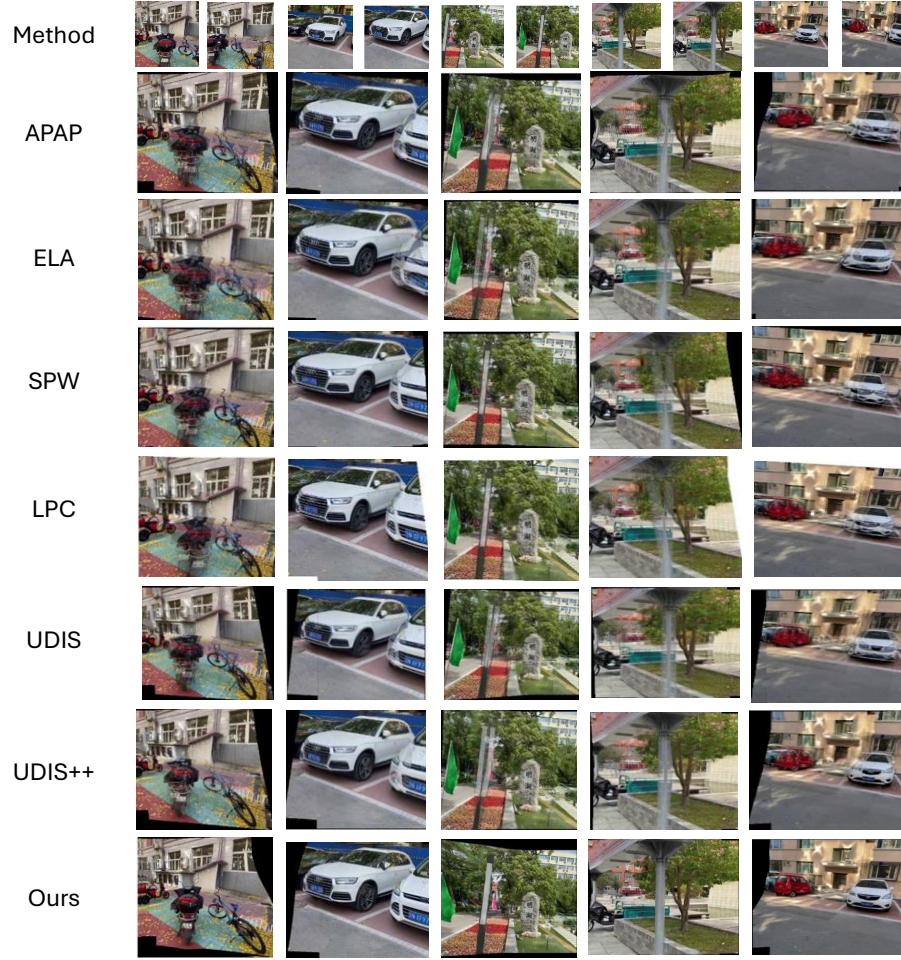
Fig. 4. We compared our image stitching results with several baselines, including APAP [36], ELA [18], SPW [20], LPC [10] [10], UDIS [27] and UDIS++ [28]. It is evident that ghosting effects are present in the results generated by the baseline methods due to misalignment of the source and target images.
