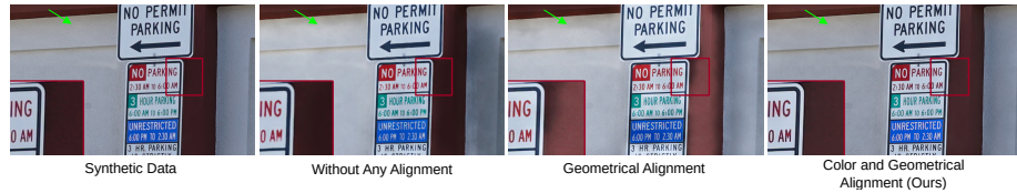
Fig. 2: The importance of Color and Geometrical Alignment between the LR and HR images for the training on Realistic SR Datasets
