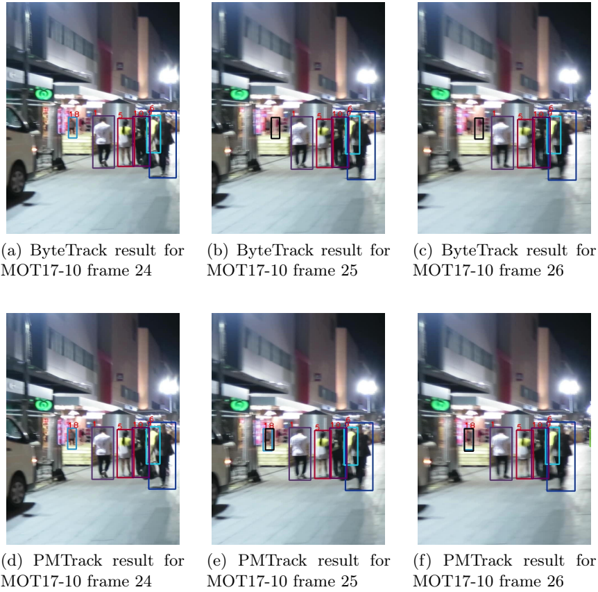
Fig. 4: Visualization of the tracking result, where the black boxes in (b) ,(c) and (e),(f) represent the predicted bounding box of the 18th tracklet. The images are from the MOT17-10 sequence.
