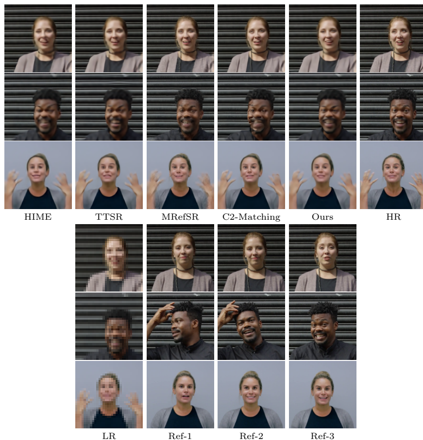
Fig. 3: Super-resolution results from the DFD test set. Here we super-resolved the low-resolution image LR with the support of high-resolution references.
