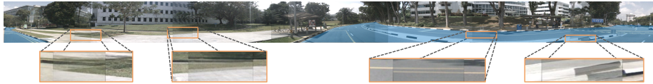
Fig. 4: Challenges in panoramic images. For example, a straight road appears curved and incomplete in the image (blue shade), distributed across different positions. Due to stitching quality issues, seams and ghosting can appear between the original adjacent images (orange boxes), causing misalignment between objects.
